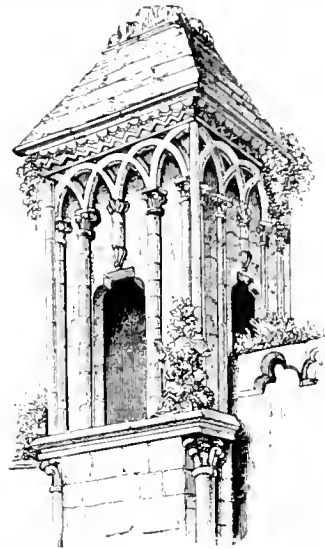
TURRET; GLASTONBURY ABBEY, C. 1200; IT COVERS THE HEAD OF A WINDING STAIR AND GIVES ACCESS TO THE ROOFS.
